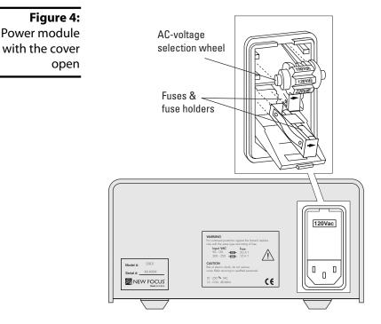
**4.** Remove the AC-voltage selection wheel from the unit.
