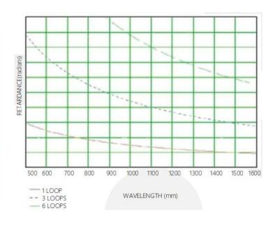
Polarization Controller's Single Paddle Delay and Wavelength, Roll relationship-(Measure unit: Fiber roll diameter 56mm, Fiber cladding diameter 125um)
