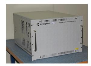
The JDS Uniphase Programmable Matrix Switch is a nonblocking, compact, rack-mountable instrument providing reliable switching operations. The design allows the user to connect any input to any output without breaking other existing connections. Standard asymmetrical (4x8, 8x12, up to 28x36) and symmetrical (8x8, 16x16, up to 32x32) configurations are offered for a broad range of applications, in standard single-mode and multimode fiber.
