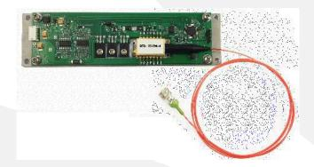
DFB-1550C-PM can be ordered as DFB- PM-M, which allows DFB laser's operating temperature and output power precisely controlled to ensure constant wavelength and power stability. It can be used for module level integration system.
